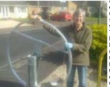
As can be seen the metal work has come galvanized, the silver colour. This will ensure it does not suffer from corrosion in the belfry. To make it look more in keeping with frame up the tower we have painted the metal work with the
